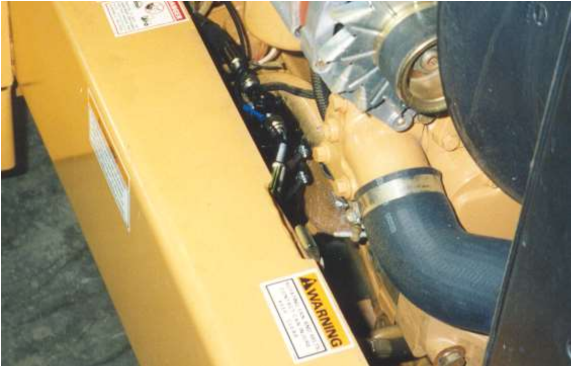
Drier in place on right side frame member.
