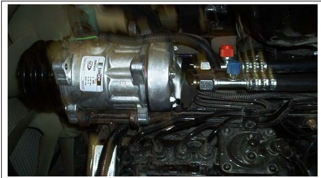
Compressor mounted showing belt and add on pulley. (Old style hose connections)
