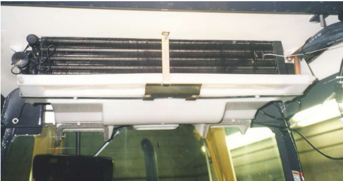
Evaporator mounted in position.
